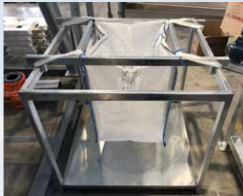
Sludge Dehydrator Bag System
